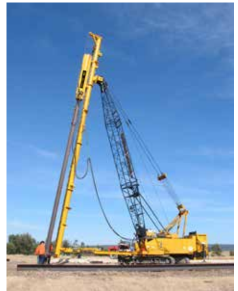
Above: The SL hammer can be used in piling rigs and is supported by a wide range of accessories.
