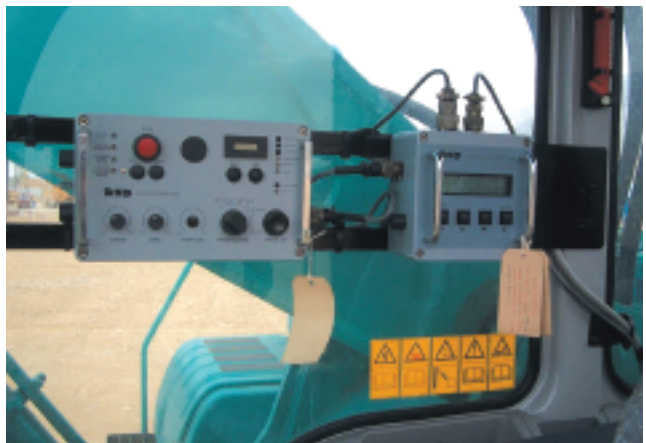
Hammer Control Box and Energy Monitoring mounted in cab
