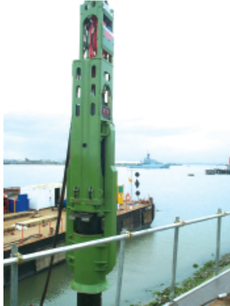
CX85, crane suspended, fitted with legs and inserts for driving steel tubular piles
