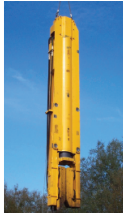
Above: Various SL30 Hammers fitted with legs and inserts for diving sheet piles. All are shown in crane suspended operation and powered by BSP Power Packs.
