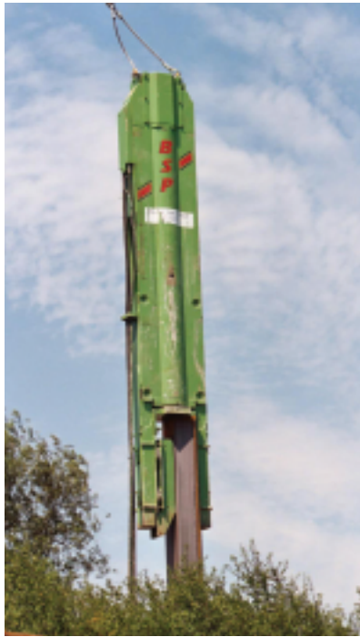
Above: Various SL30 Hammers fitted with legs and inserts for diving sheet piles. All are shown in crane suspended operation and powered by BSP Power Packs.
